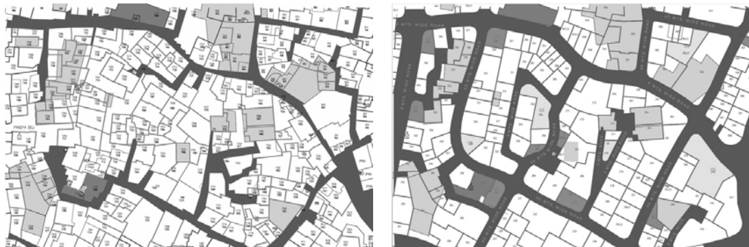
Figure 24: Land re-adjustment in Bhuj: Map of a neighborhood in the old city urban core area of Bhuj shows plot lines and road layout before (top left) and after (top right) land re-adjustment. (Source: Maps provided by Environmental Planning Collaborative, Ahmedabad)
